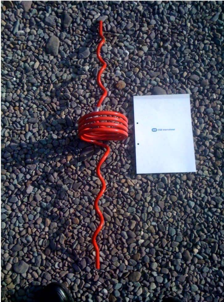
Figure 14.1 Spiral type bird flight diverter proposed for use at the crossing of Owenbeg River at Boleybeg
